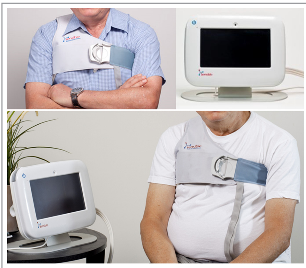
Figure 1. Remote dielectric sensing system: a vest and monitor to show data.
